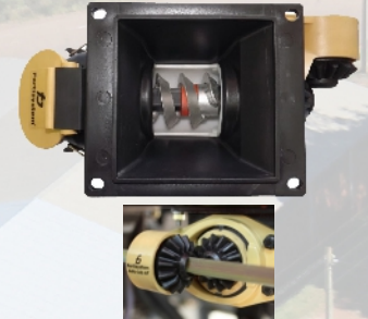
Fertilizer distribution system FertiSystem AGRIMAC
